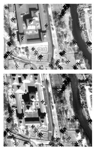
Figure 4. Example of matching QuickBird stereo images. The matched points are labelled by black crosses.
