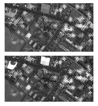
Figure 2. Image matching for the registration of IKONOS stereo images of Hobart, Australia.
